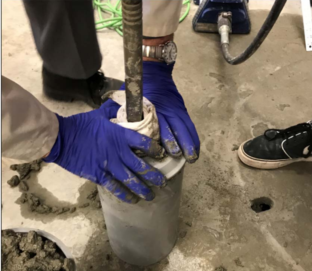
Figure 1.6. Sample vibrating with cap to prevent air voids getting into system
